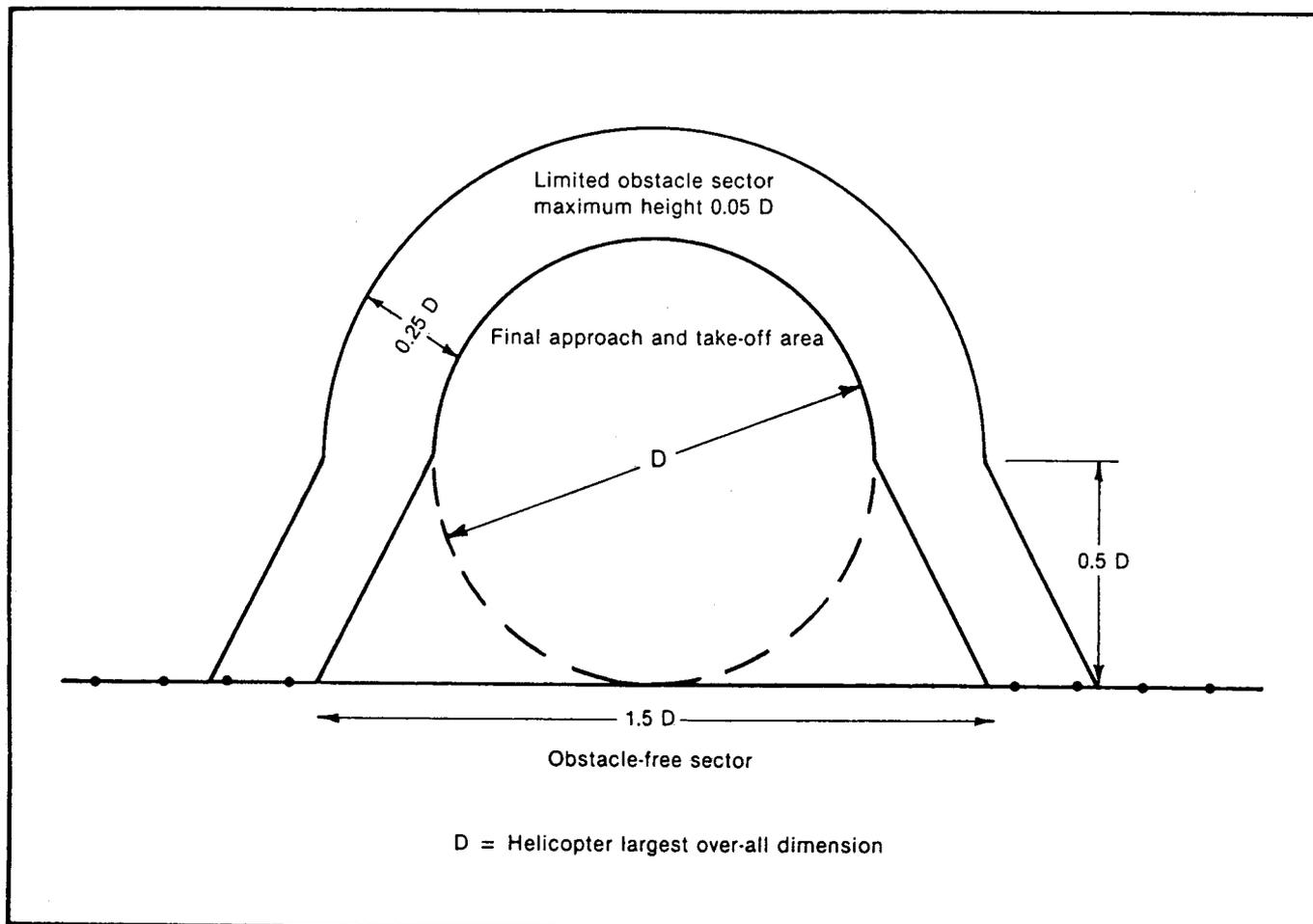
Figure 4-12. Ships-side non-purpose built heliport
