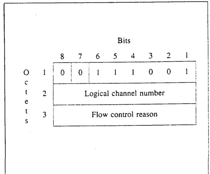
Figure 4-24. Flow control (resume) SNMPDU format
