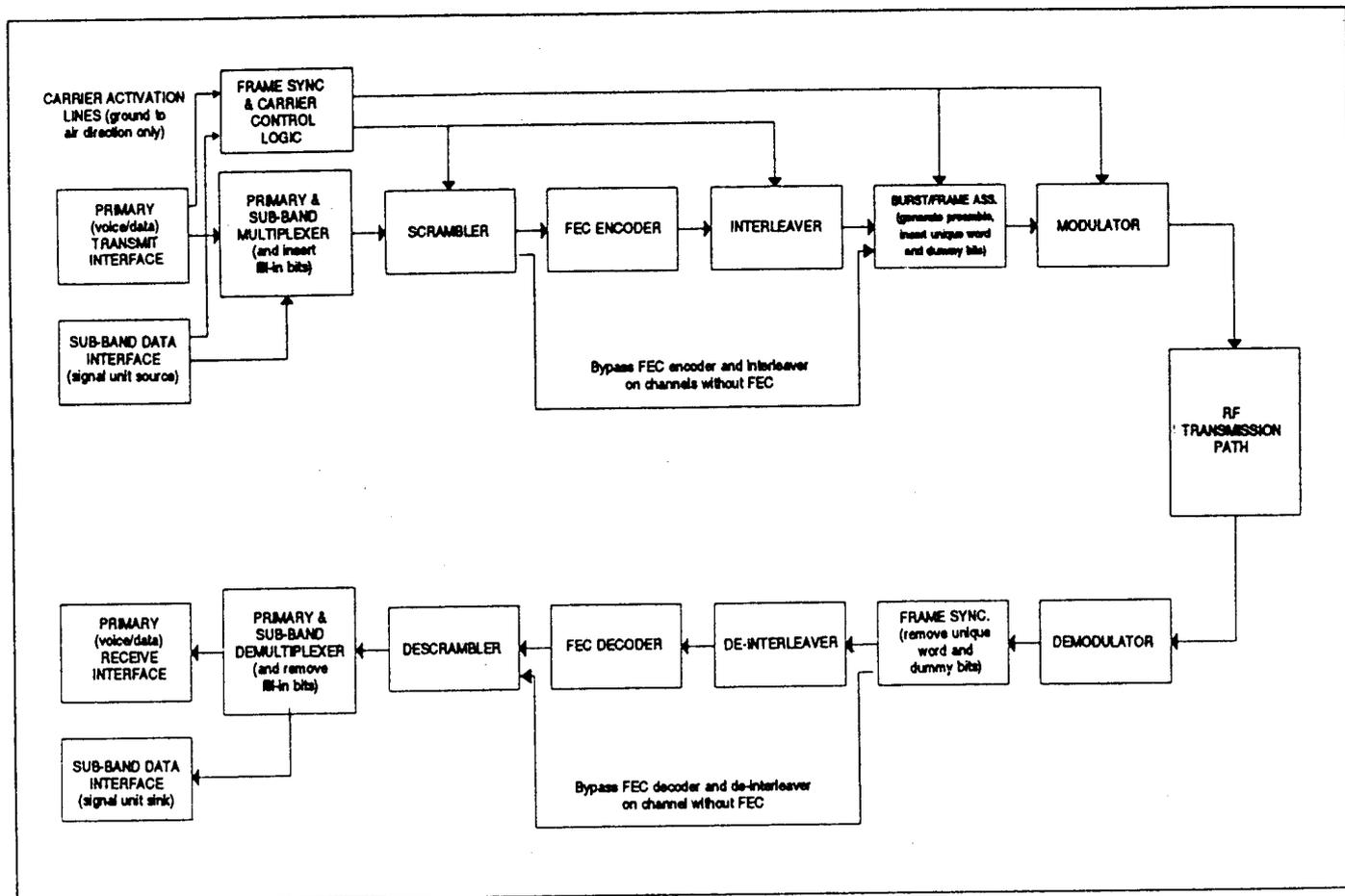
Figure A-13. C channel functional blocks
