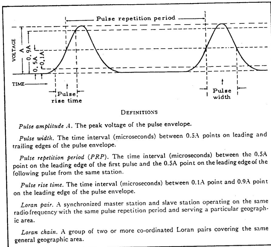
**Figure 3-4. Loran-A pulse shape and spacing definitions**
