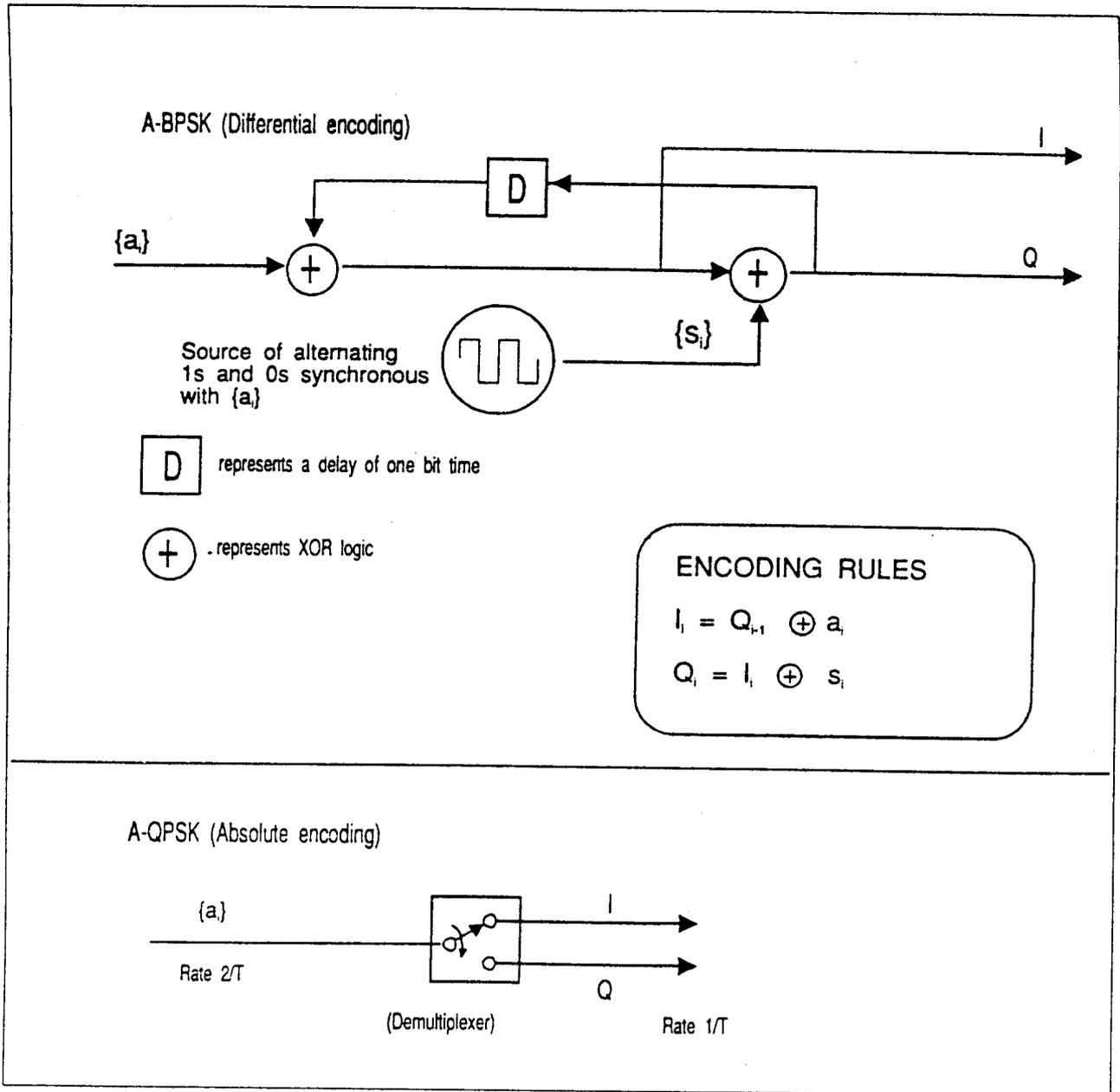
Figure A-3. Data encoders for modulator model
