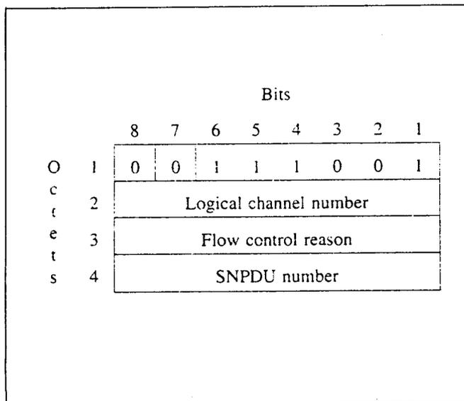
Figure 4-23. Flow control (suspend) SNMPDU format
