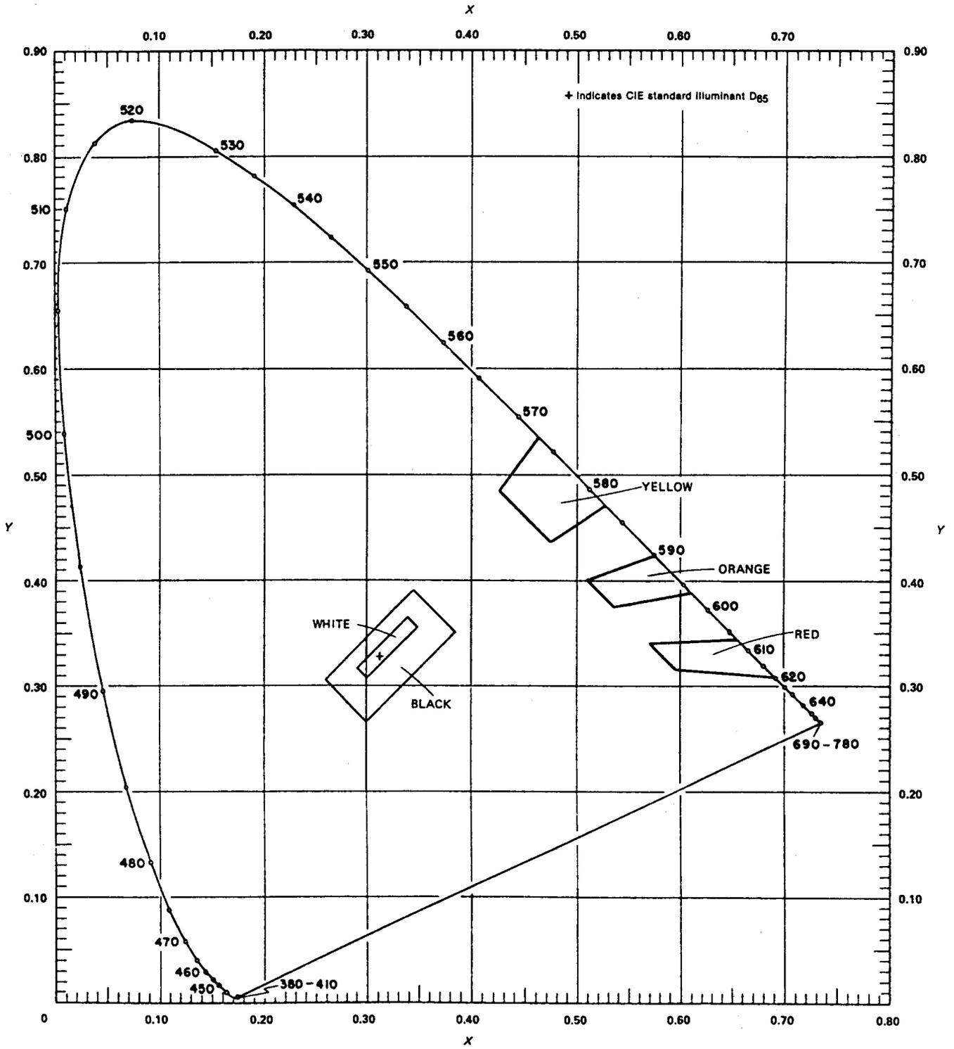
Figure 1.2 Ordinary colours for surface markings
