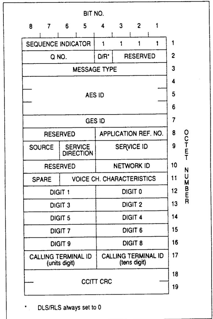
Figure A2-46. Abbreviated access request telephone — R channel
