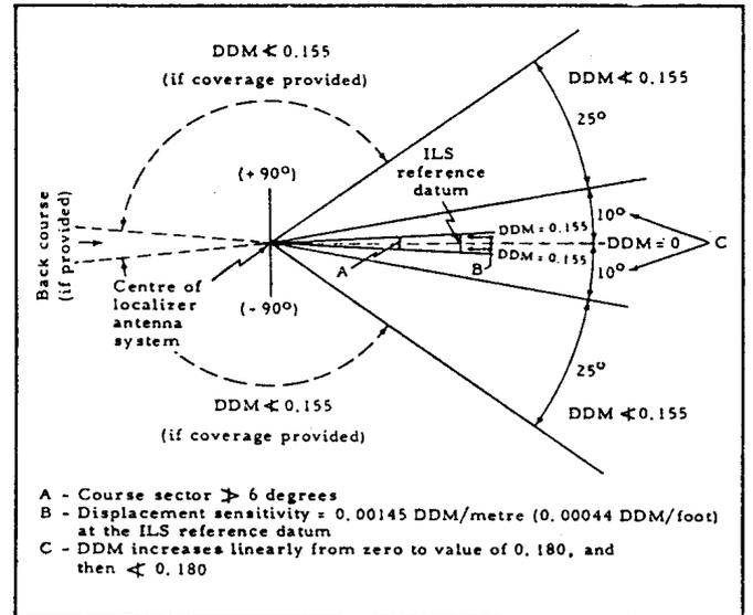
Figure C-9. Difference in depth of modulation and displacement sensitivity
