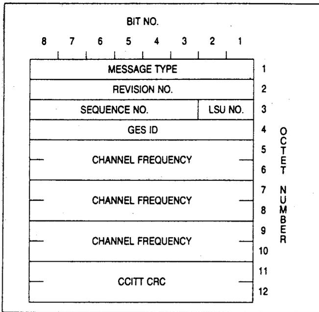
Figure A2-31. AES system table broadcast — P channel
