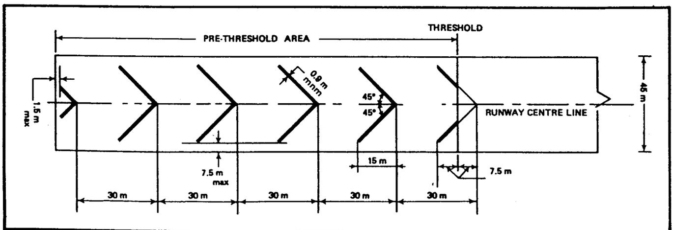
Figure 7-2. Pre-threshold marking
