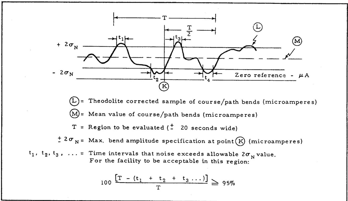
Figure C-2. Evaluation of course/path bend amplitude
