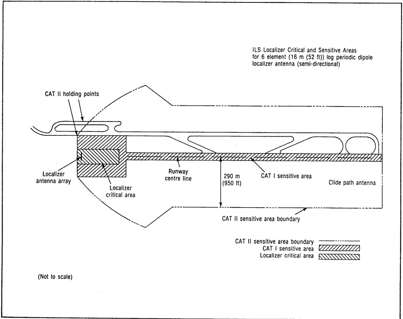
Figure C-4A. Example of critical and sensitive area application at specific sites with 747 aircraft interference
