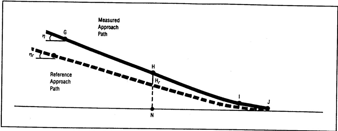
Figure 1-8. Comparison of measured and corrected approach profiles
