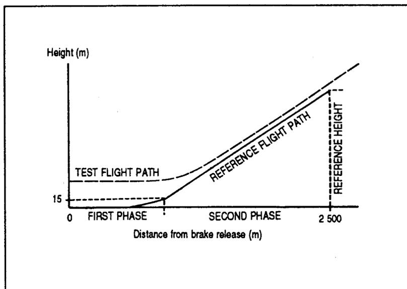
Figure 6-1. Typical test and reference profiles
