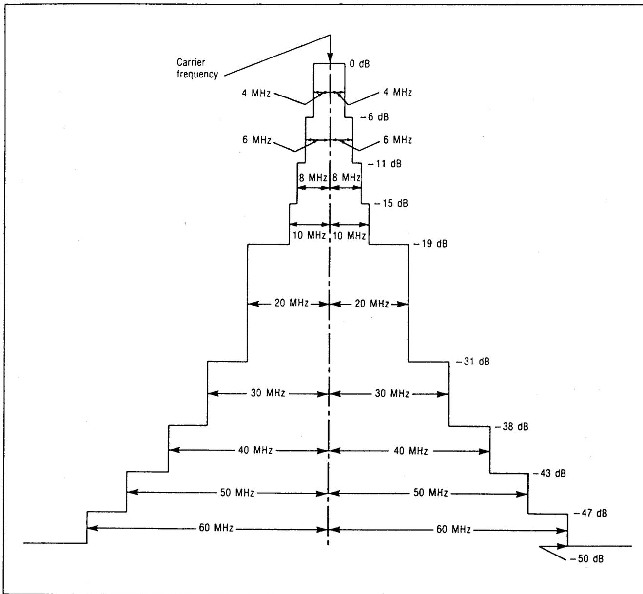
Figure 3-3.1. Required spectrum limits for interrogator transmitter
