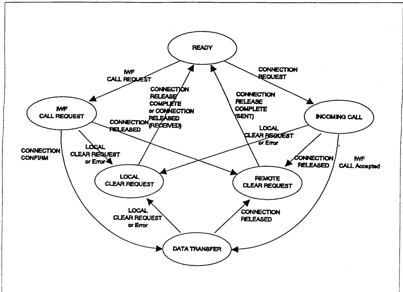
Figure 4-29. Connection establishment and release state diagram
