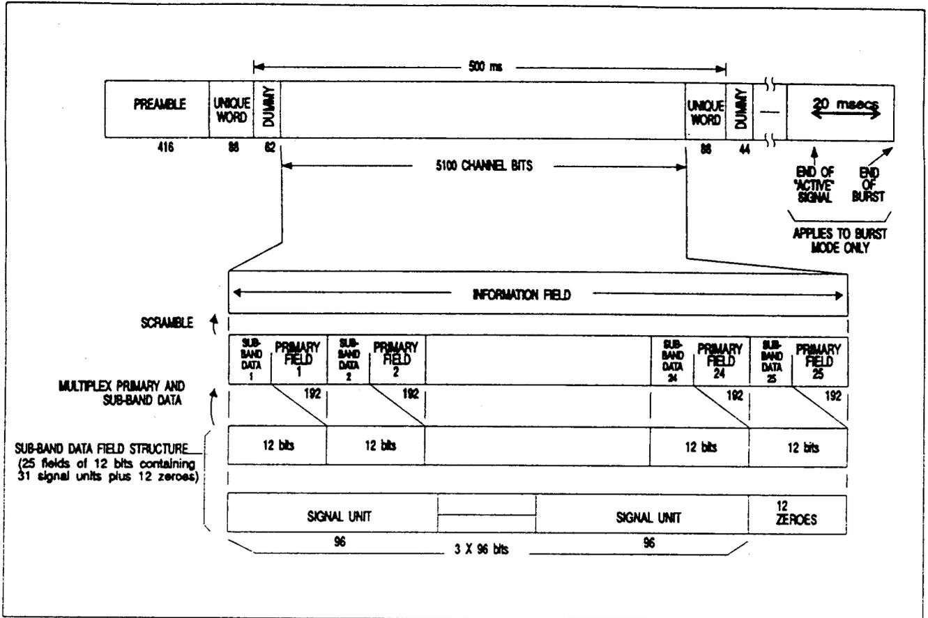
Figure 4-10. C channel format at 10.5 kbits/s channel rate
