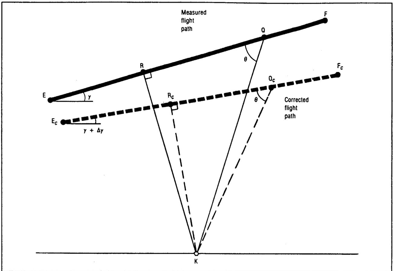
Figure 1-6. Take-off profile characteristics influencing sound level
