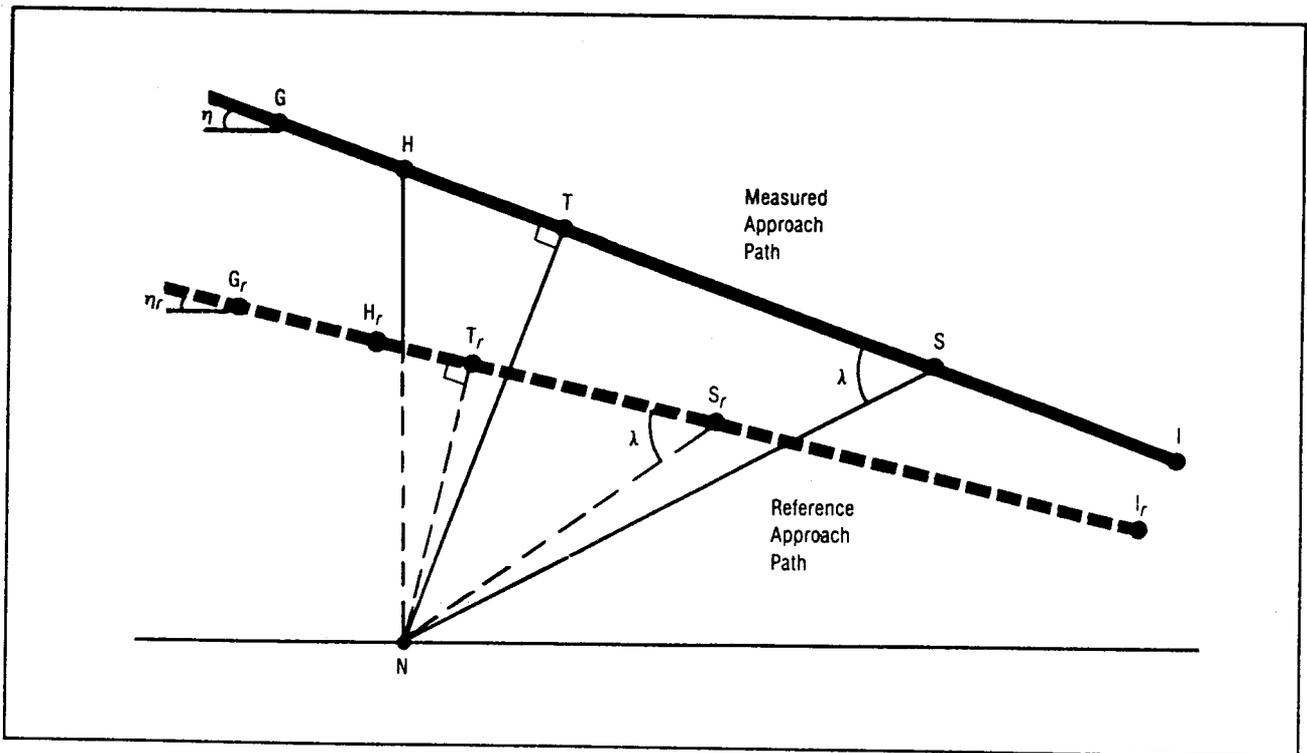
Figure 1-9. Approach profile characteristics influencing sound level
