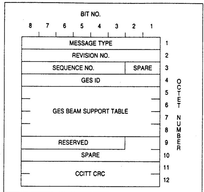
**Figure A2-60. AES system table broadcast — P channel**
