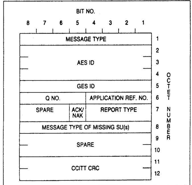
Figure A2-26. Telephony acknowledgement — P/sub-band C channel
