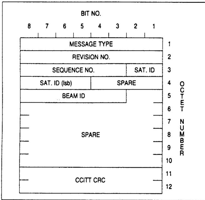
**Figure A2-59. AES system table broadcast — P channel**
