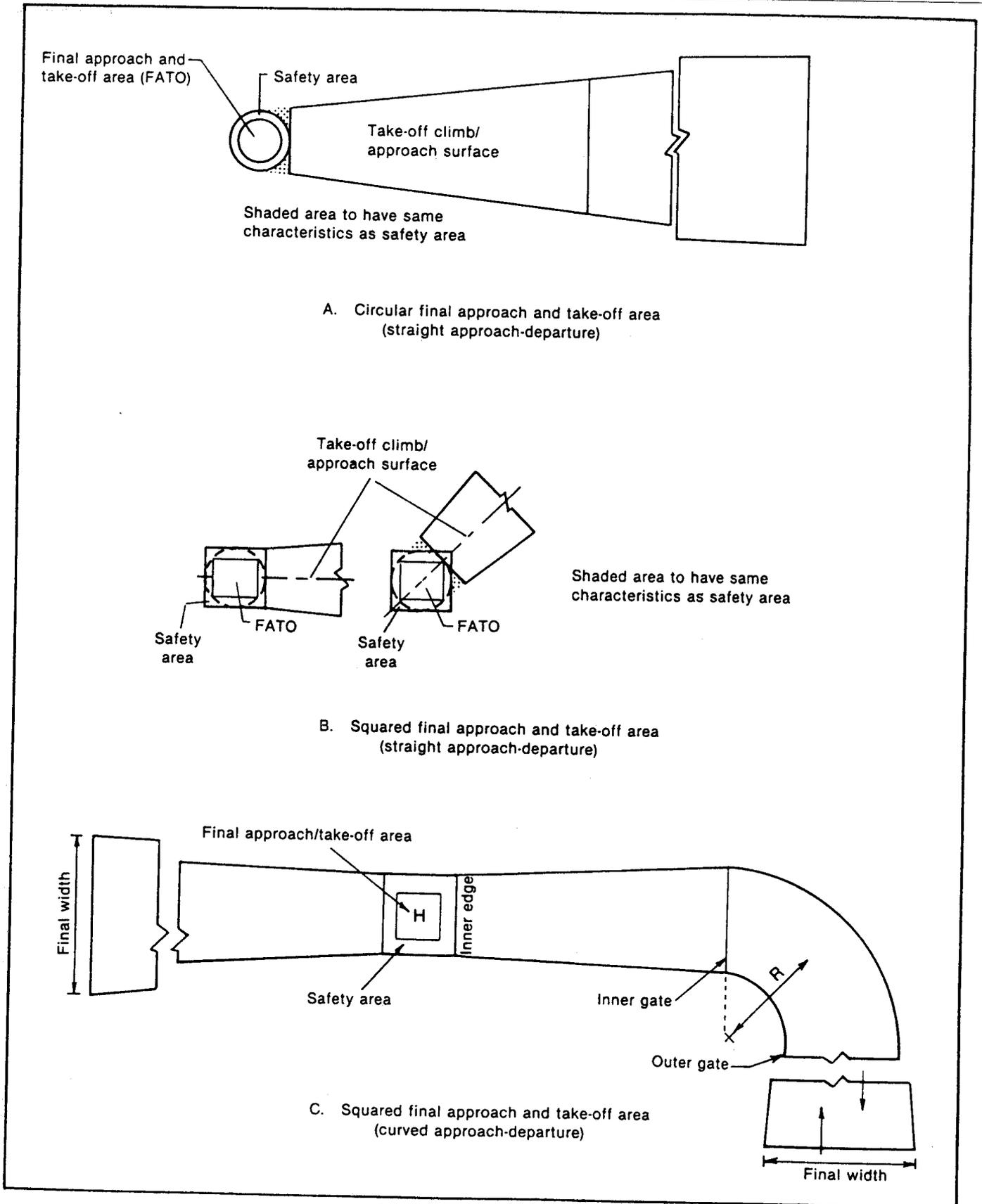
Figure 4-6. Take-off climb/approach surface (non-instrument FATO)
