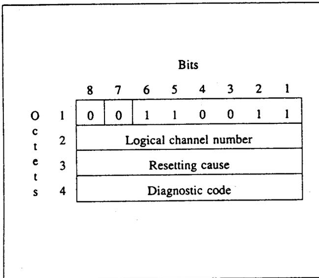
Figure 4-21. Reset SNMPDU format
