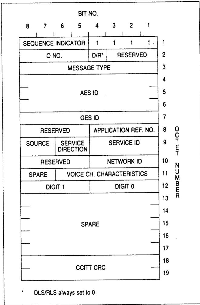
Figure A2-45. Access request telephone — R channel
