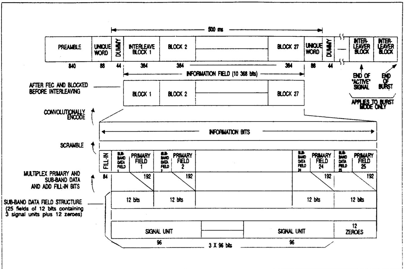
Figure 4-9. C channel format at 21.0 kbits/s channel rate
