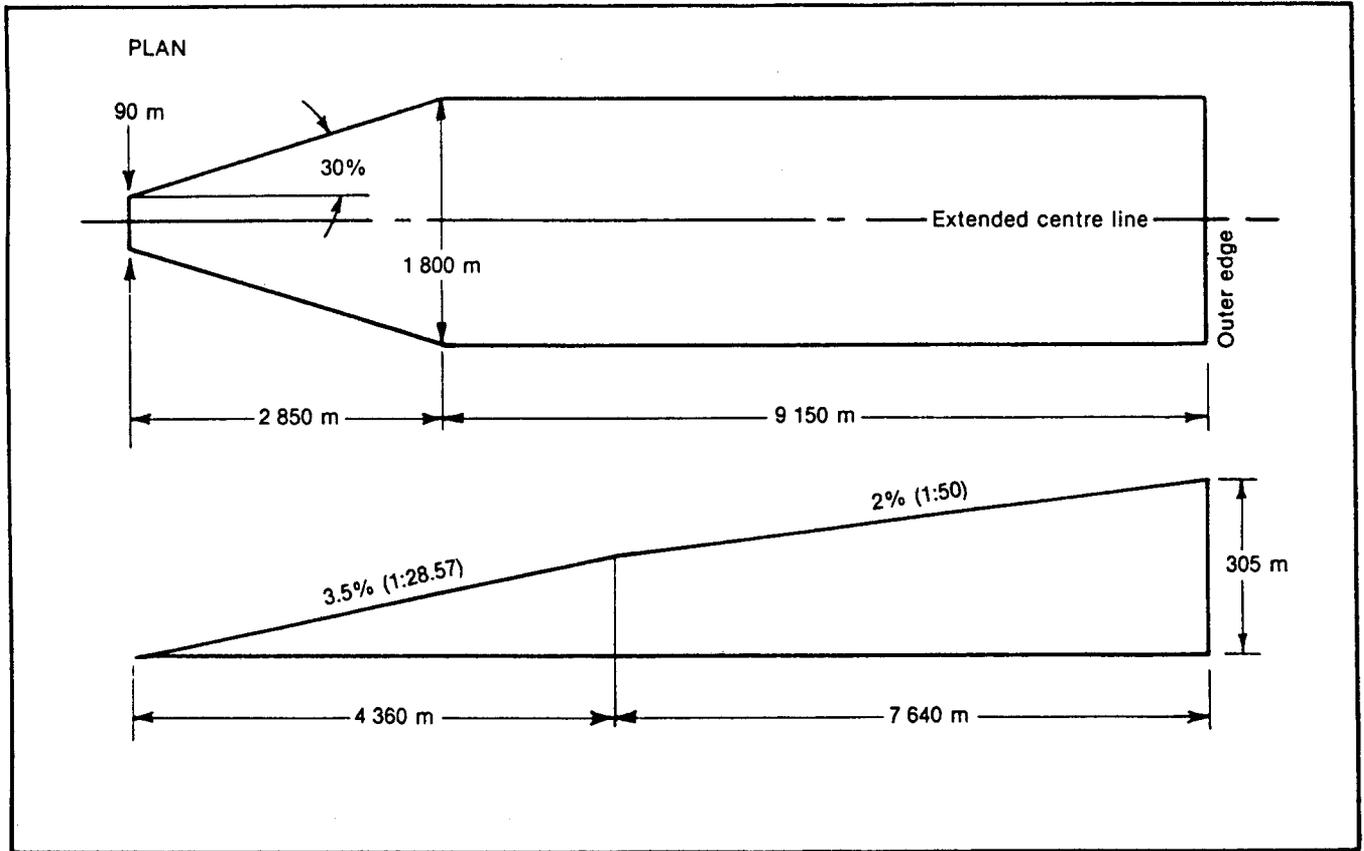
Figure 4-7. Take-off climb surface for instrument FATO
