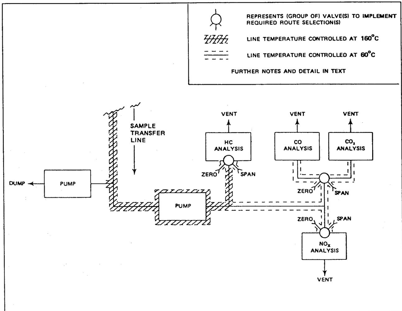
Figure 5-2. Sample transfer and analysis system, schematic
