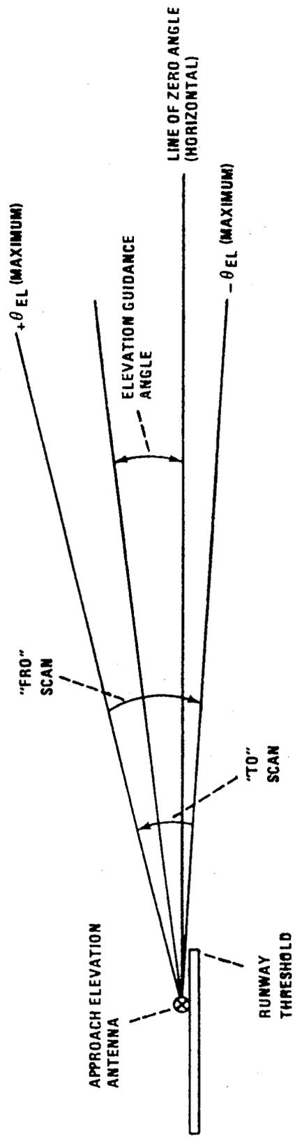
Figure G-7. Scanning conventions for approach elevation and flare guidance functions
