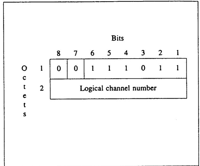
Figure 4-22. Reset confirm SNMPDU format
