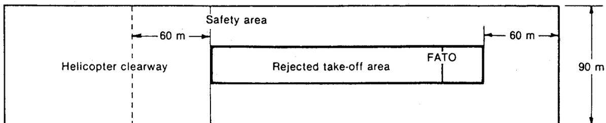
Figure 3-1. Safety area for instrument FATO
