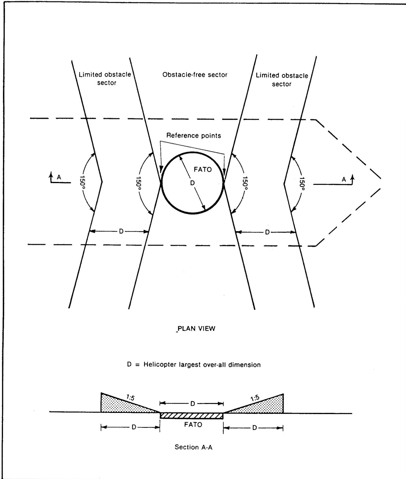
Figure 4-11. Midship non-purpose built heliport obstacle limitation surfaces
