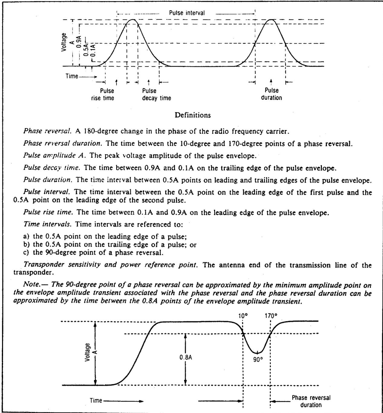
**Figure 3-3. Definitions of secondary surveillance radar waveform shapes, intervals and the reference point for sensitivity and power**
