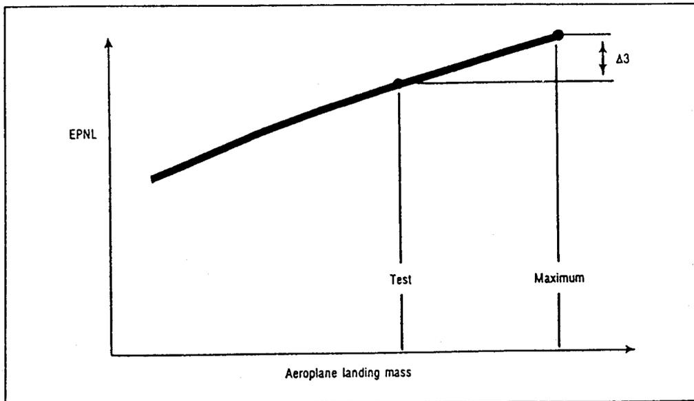
Figure 1-11. Approach mass correction for EPNL
