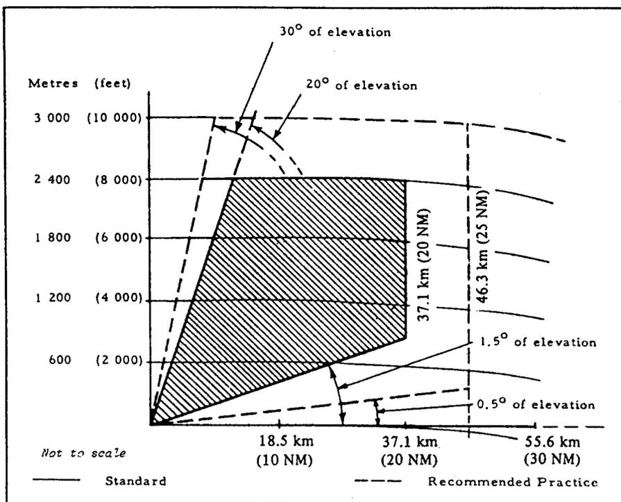
Figure C-18. SRE of precision approach radar system — Vertical coverage on a 15 m<sup>2</sup> echoing area aircraft
