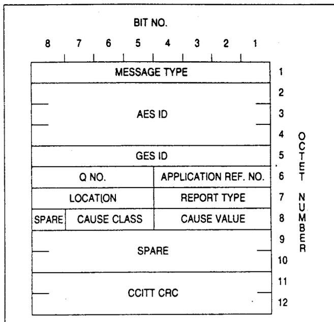
Figure A2-16. Call progress — P or to-/from-aircraft sub-band C channel
