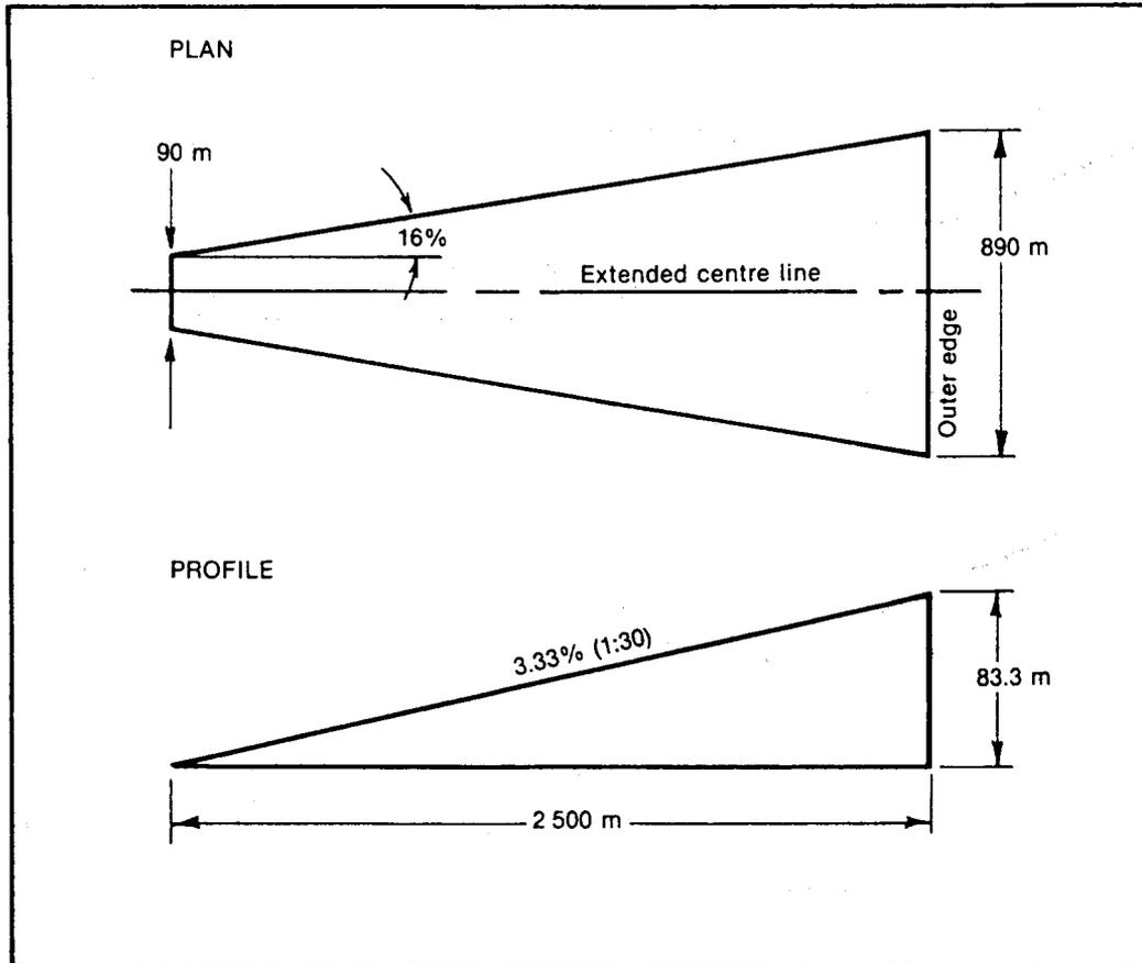
Figure 4-9. Approach surface for non-precision approach FATO
