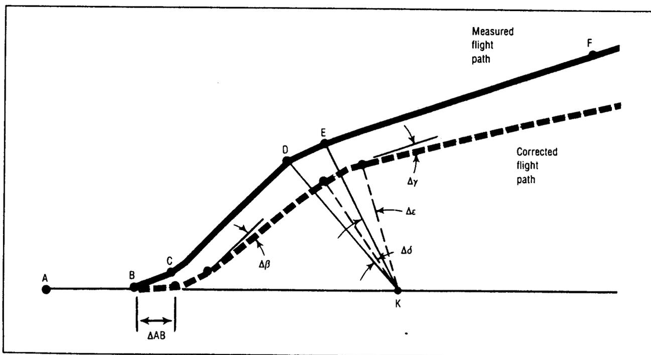
Figure 1-5. Comparison of measured and corrected take-off profiles
