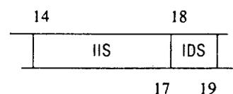
The following subfields shall be inserted by the transponder into the UM field of the reply if a surveillance or Comm-A interrogation (UF equals 4, 5, 20, 21) contains DI = 1 and RSS other than zero:
