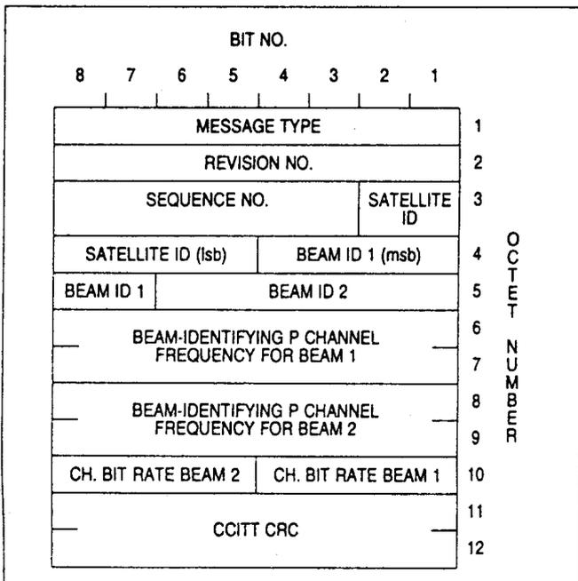
Figure A2-33. AES system table broadcast — P channel
