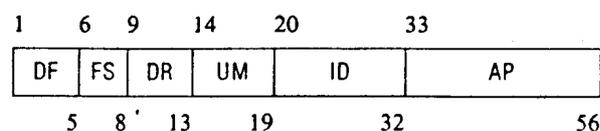
This reply shall be generated in response to an interrogation UF 5 or 21 with an RR field value less than 16. The format of this reply shall consist of these fields:
