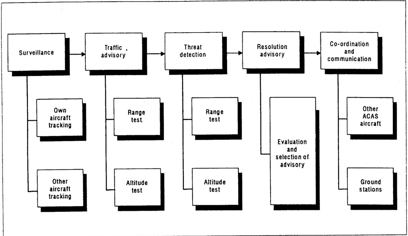
Figure A-1. Illustration of ACAS functions
