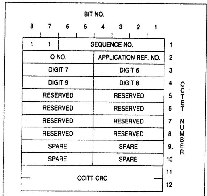
Figure A2-10. Call information telephone — from-aircraft sub-band C channel
