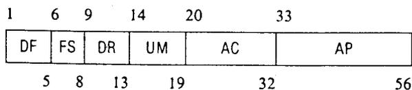
This reply shall be generated in response to an interrogation UF 4 or 20 with an RR field value less than 16.
