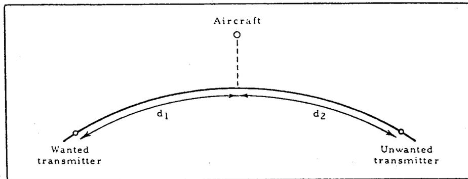
Figure A-6. VOLMET planning (illustrating adjacent channel protection)
