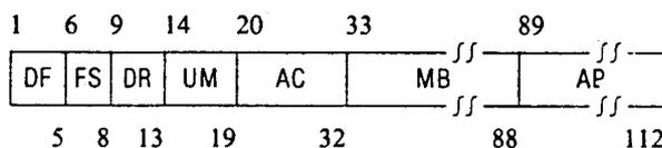
This reply shall be generated in response to an interrogation UF 4 or 20 with an RR field value greater than 15. The format of this reply shall consist of these fields:
