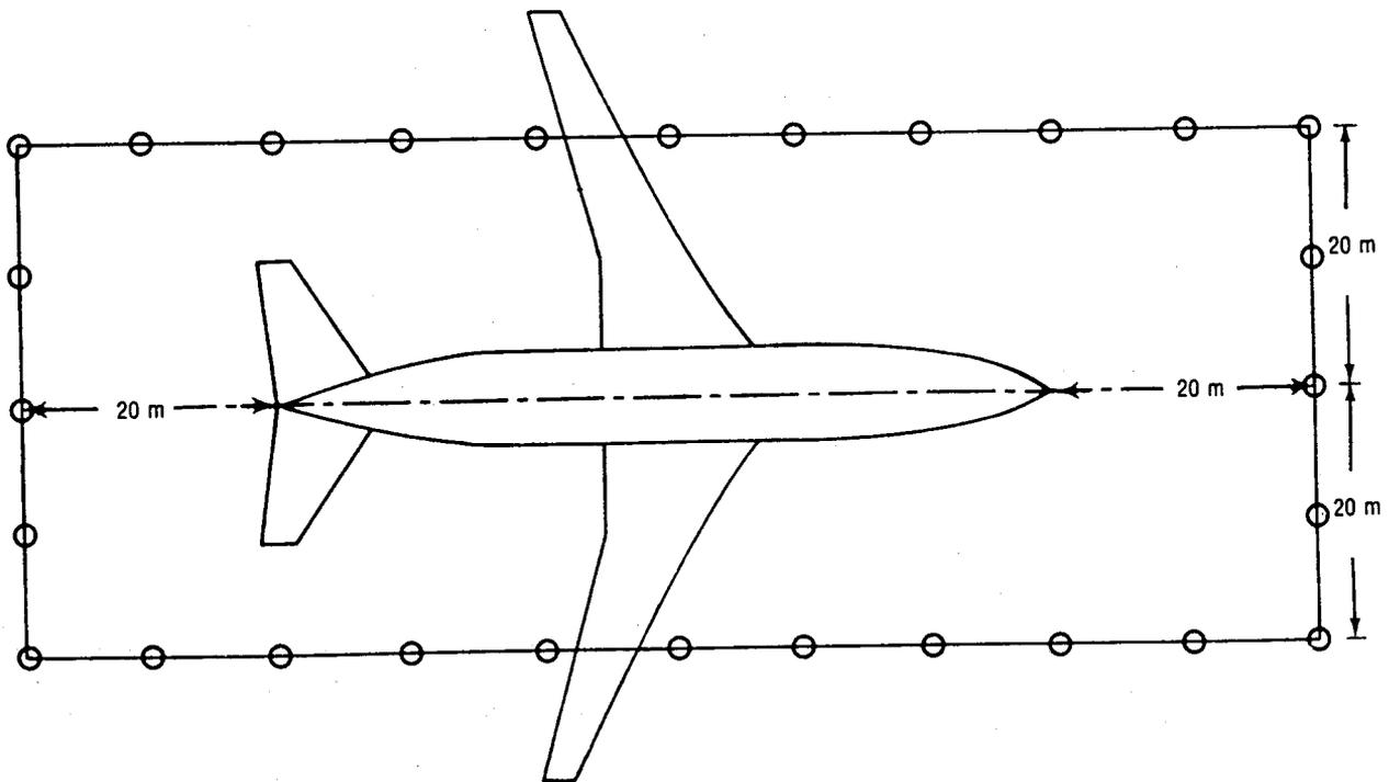
Figure C-2. Rectangle of noise survey measurement positions
