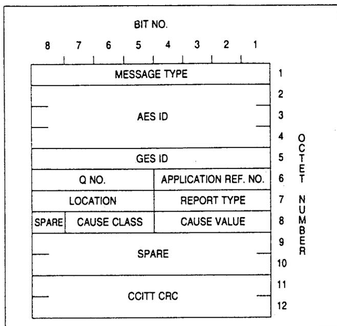
Figure A2-15. Call progress — P or to-/from-aircraft sub-band C channel
