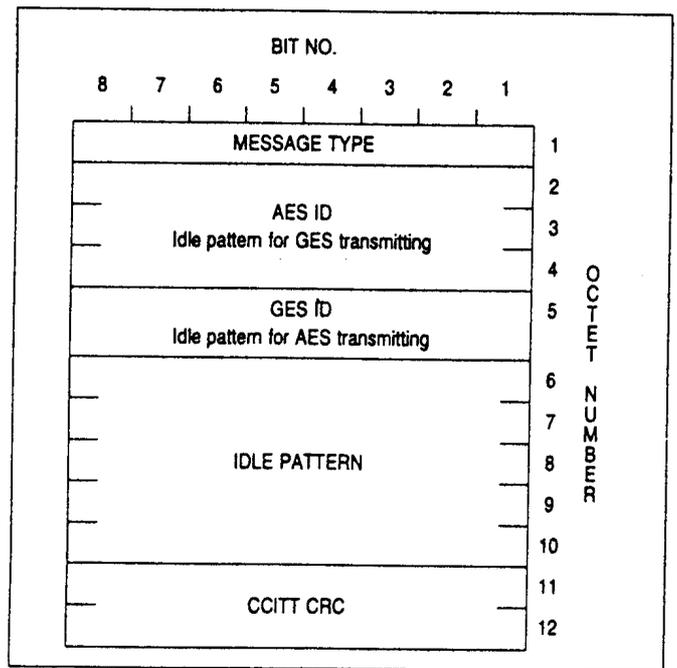
Figure A2-42. Fill-in — P, T and to-/from-aircraft
