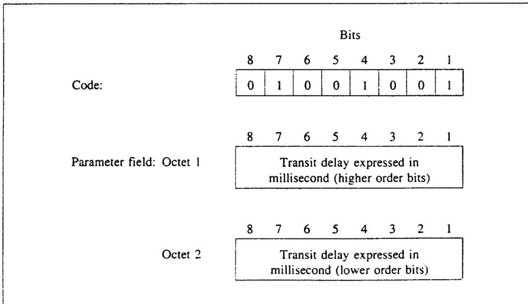
Figure 4.26. Transit delay selection and indication facility format
