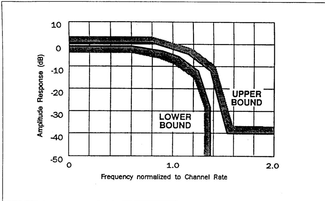
Figure A-5. AES A-BPSK transmit filter response mask
