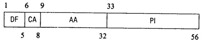
The reply to the Mode S-only all-call or the Mode A/C/S all-call interrogation shall be the Mode S all-call reply, downlink format 11. The format of this reply shall consist of these fields:
