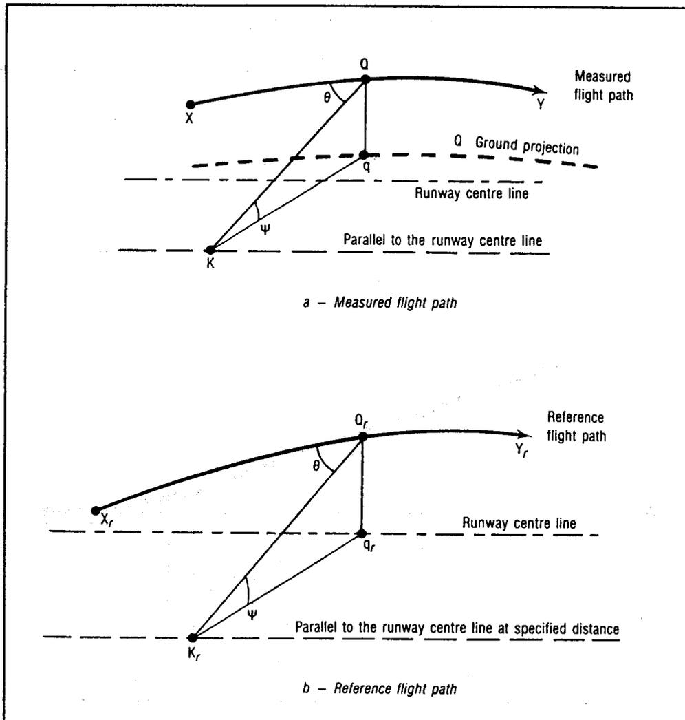
Figure 2-11. Lateral measurement — determination of reference station
