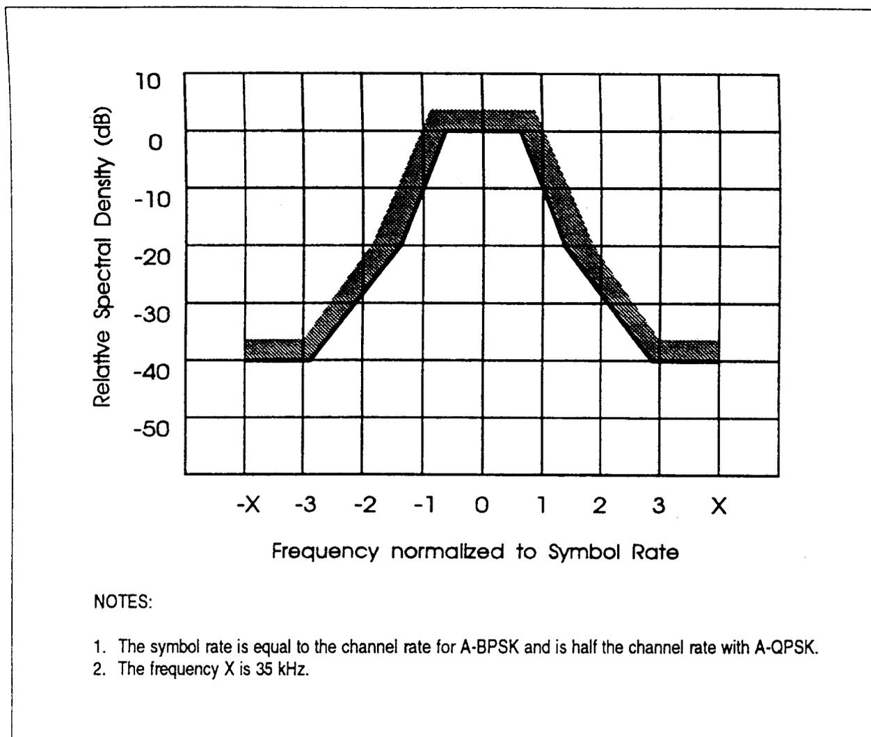
Figure A-8. Required spectral limits for AES transmissions
