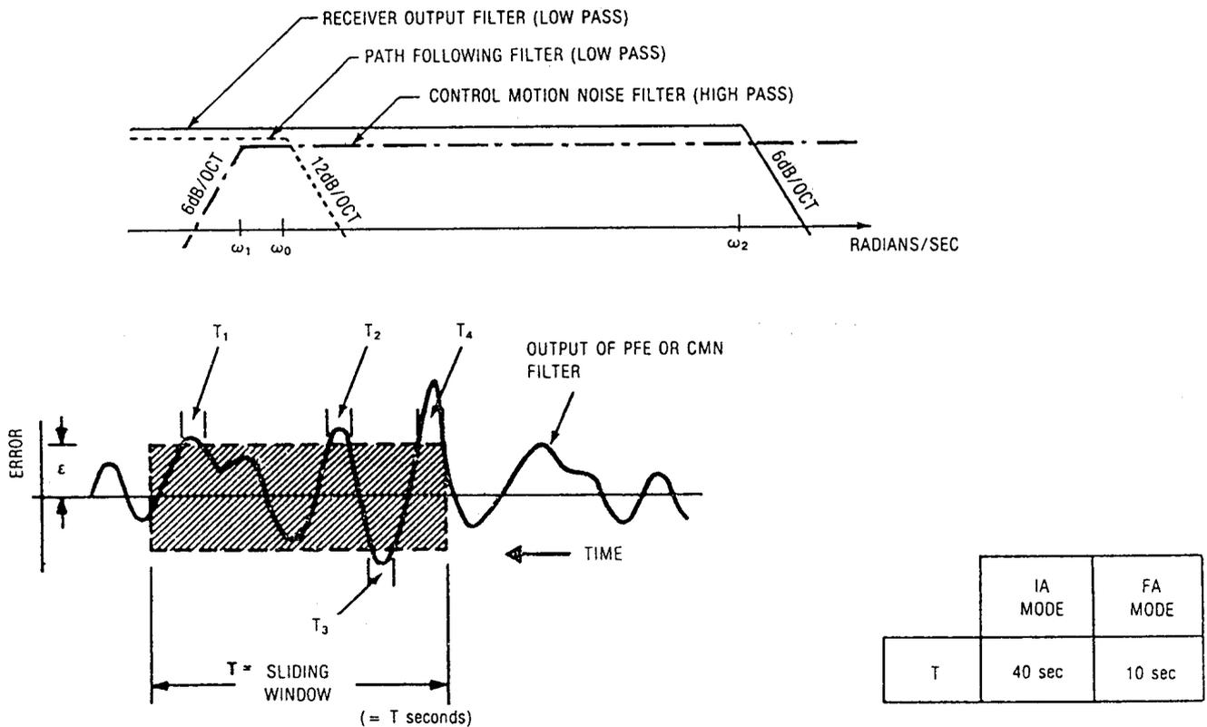
DME/P measurement methodology.  $\epsilon$  is the error specification; T region to be evaluated;  $T_1, T_2, T_3, \dots$  time intervals that error exceeds specifications. For the equipment to be acceptable in this region, the following inequality should be true:  $(T_1 + T_2 + T_3 + \dots) / T \leq 0.05$ .
