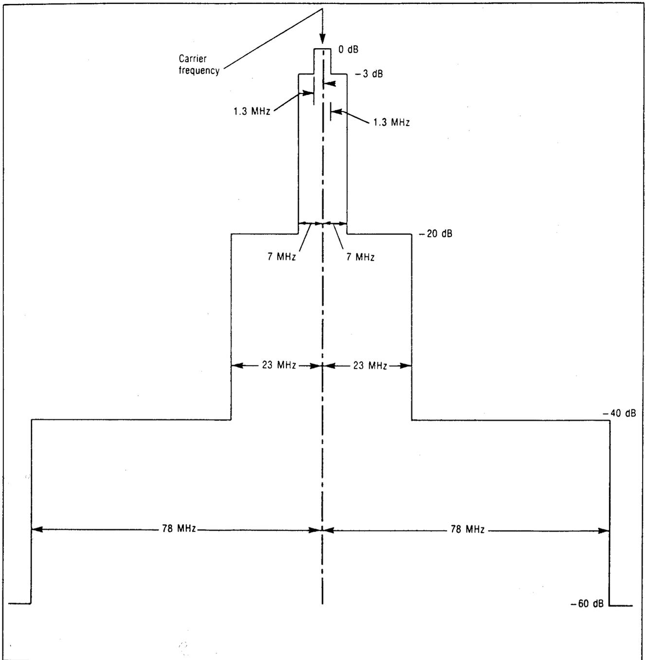
Figure 3-3.4. Required spectrum limits for transponder transmitter
