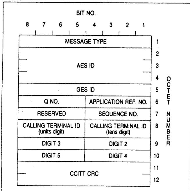
Figure A2-9. Call information telephone — from-aircraft sub-band C channel
