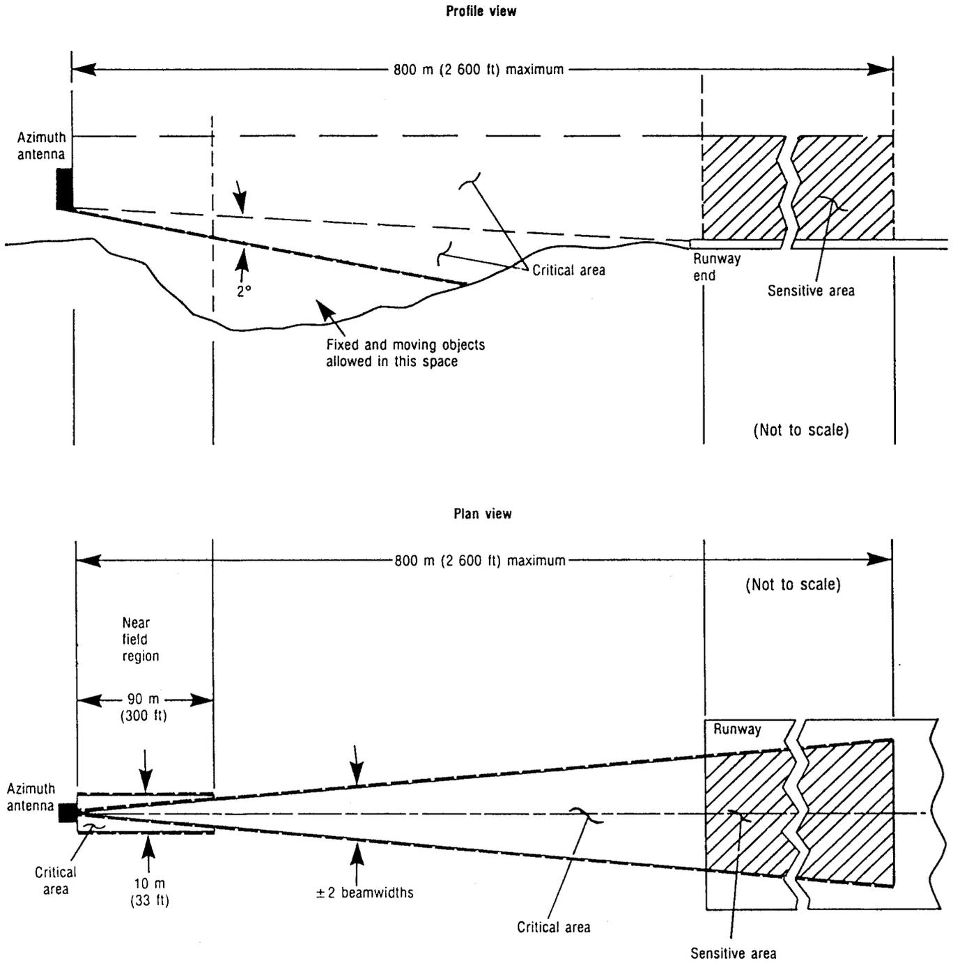
Figure G-17. Typical azimuth critical and sensitive areas
