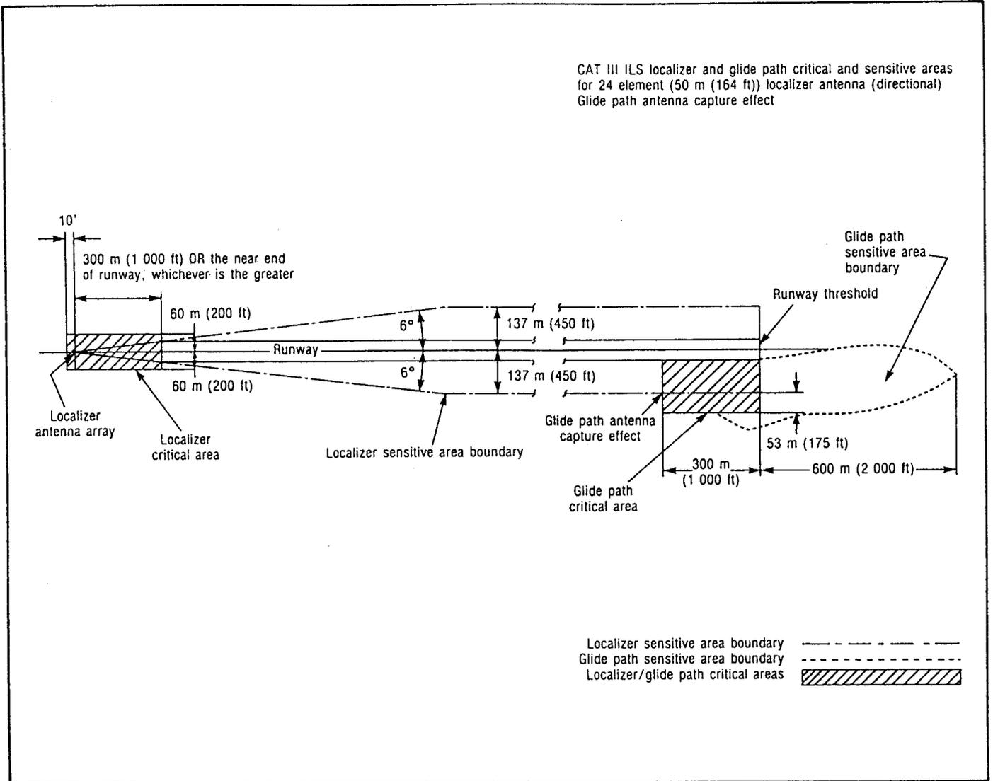
Figure C-4B. Example of critical and sensitive area application at specific sites with 747 aircraft interference
