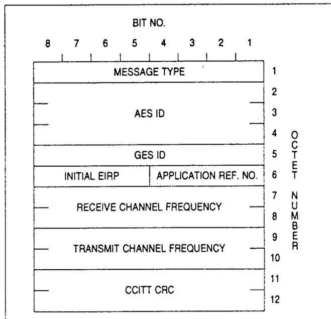
Figure A2-17. C channel assignment — P channel
