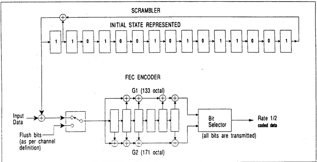
Figure 4-3. Scrambler and convolutional encoder functions
