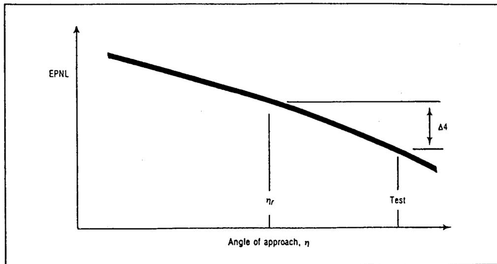
Figure 1-12. Approach angle correction for EPNL
