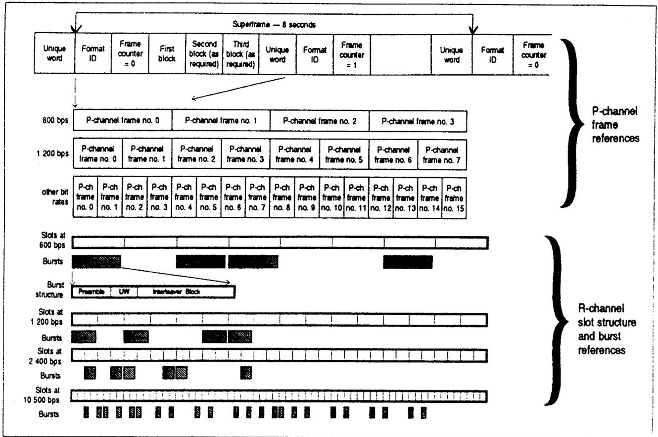
Figure 4-5. Timing references between P and R channels
