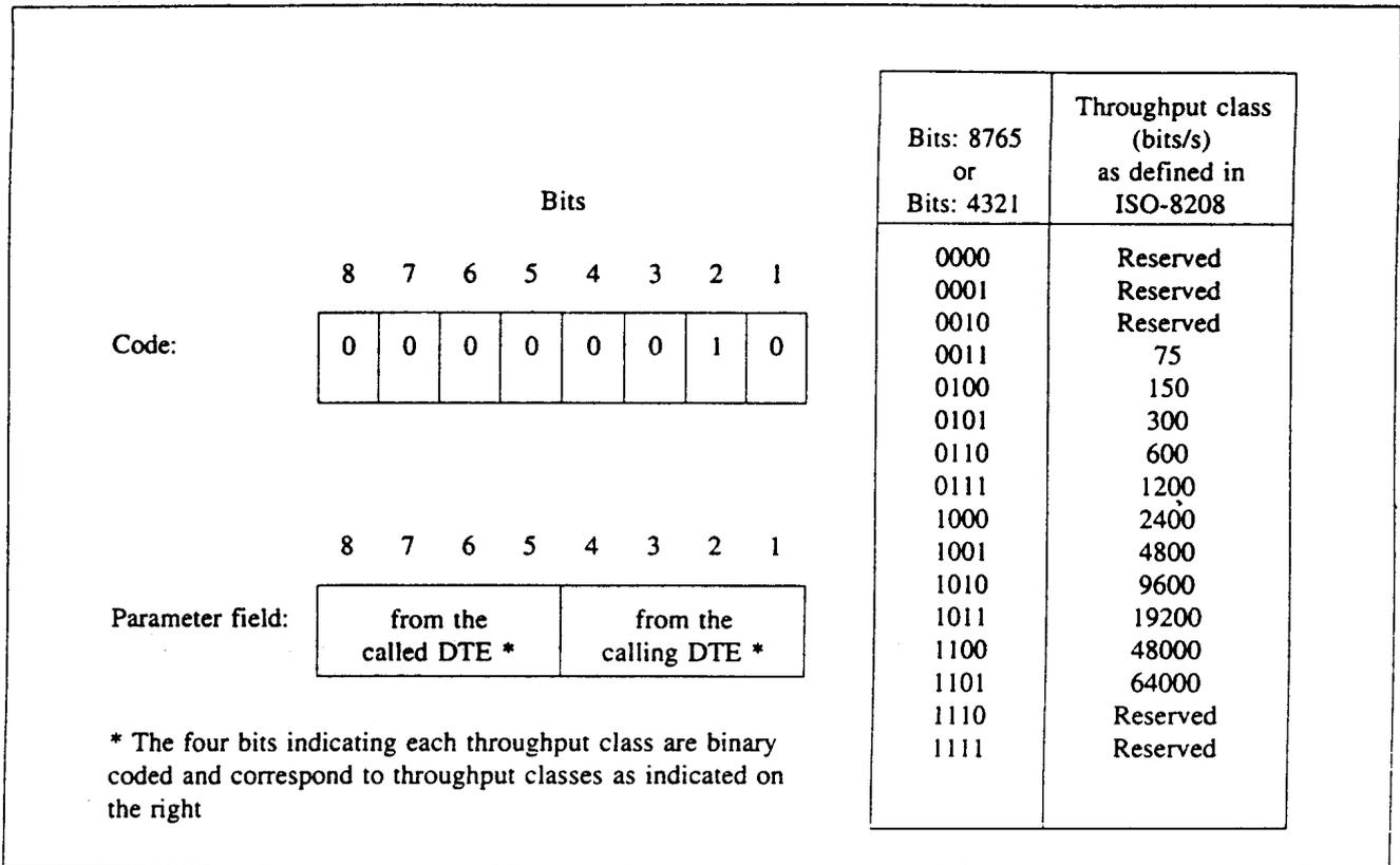
Figure 4-25. Throughput class negotiation (TCN) facility field
