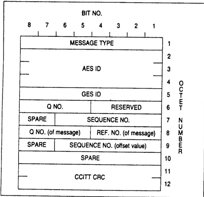
Figure A2-41. Retransmission header —
