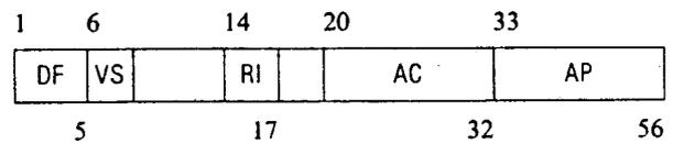
This reply shall be sent in response to an interrogation with UF equals zero and RL equals zero. The format of this reply shall consist of these fields:
