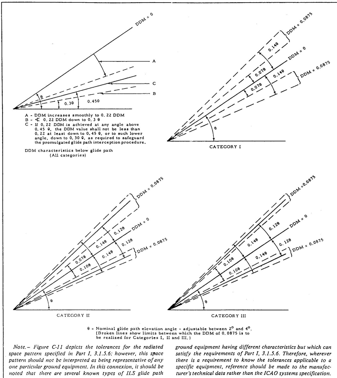
Figure C-11. Glide path — Difference in depth of modulation
