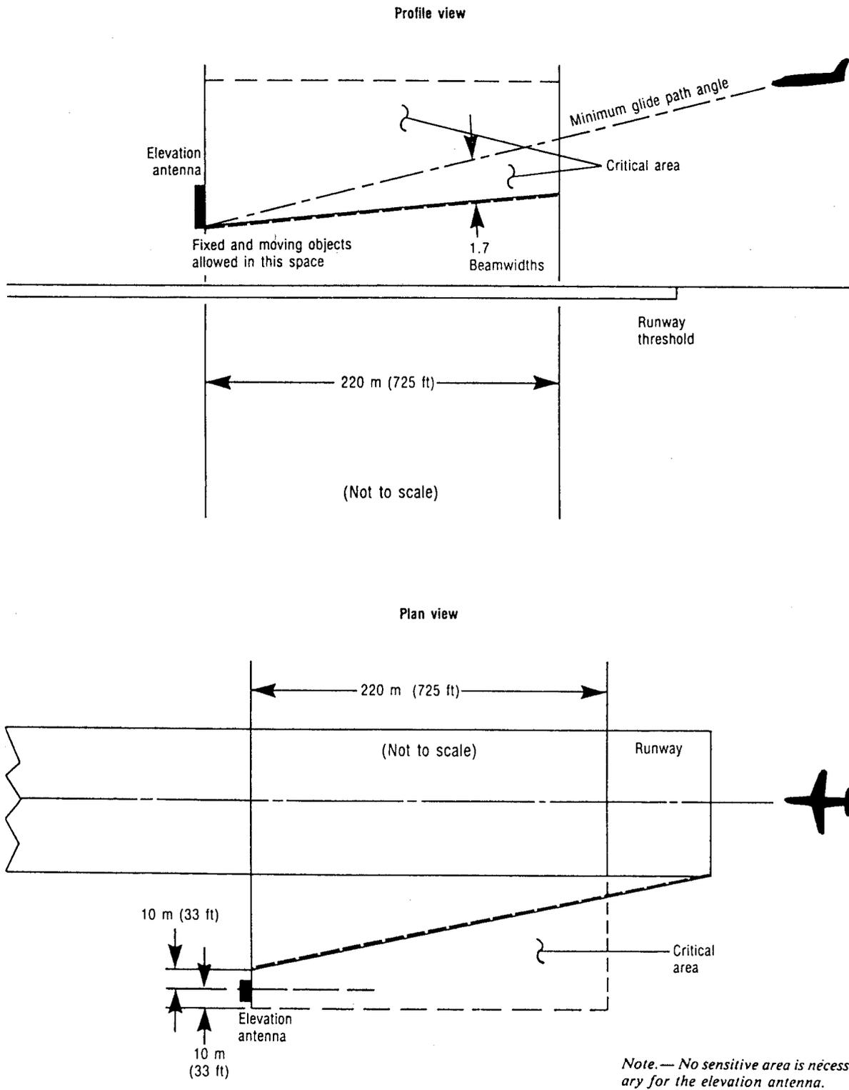
Figure G-18. Typical elevation critical area
