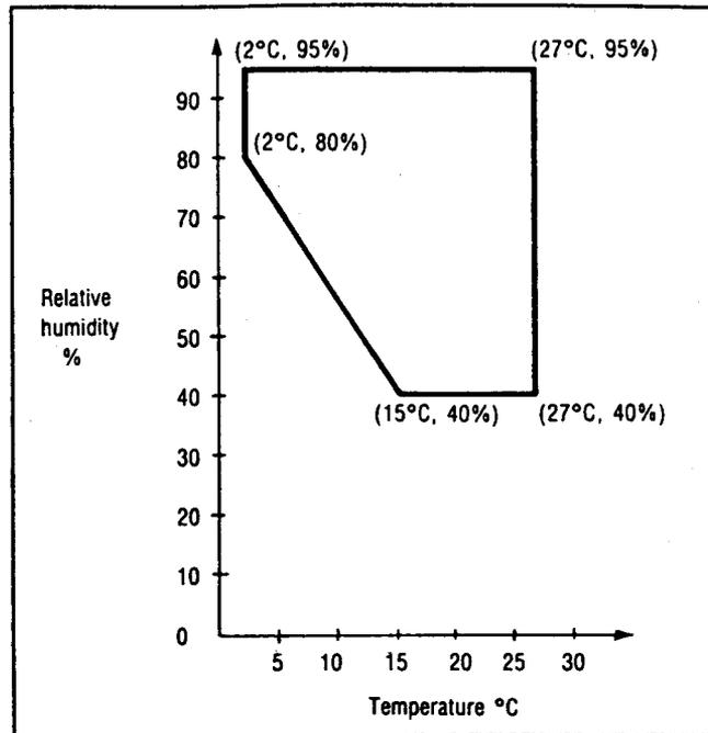
Figure 6-2. Measurement window for no absorption correction
