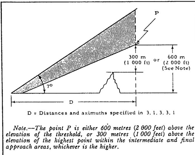
Figure C-8. Localizer coverage with respect to elevation
