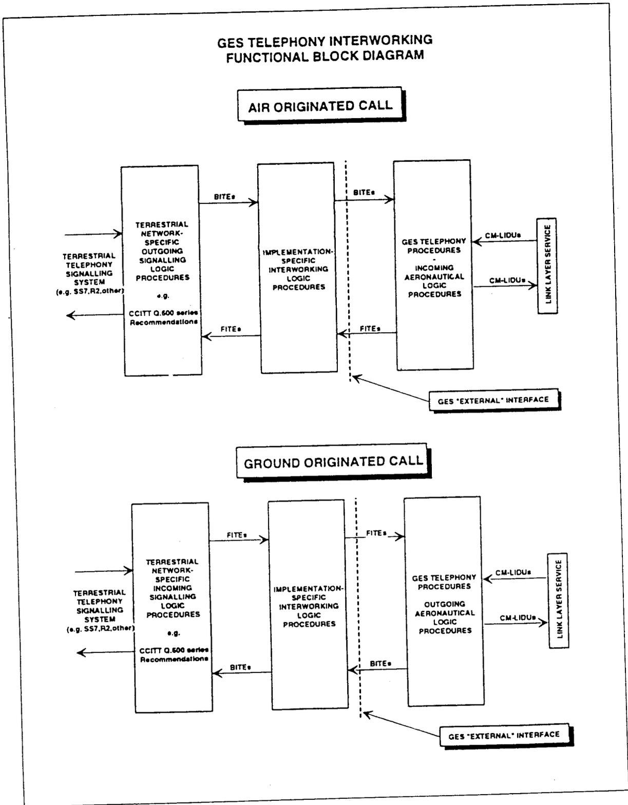
Figure A-19. GES telephony interworking block diagram
