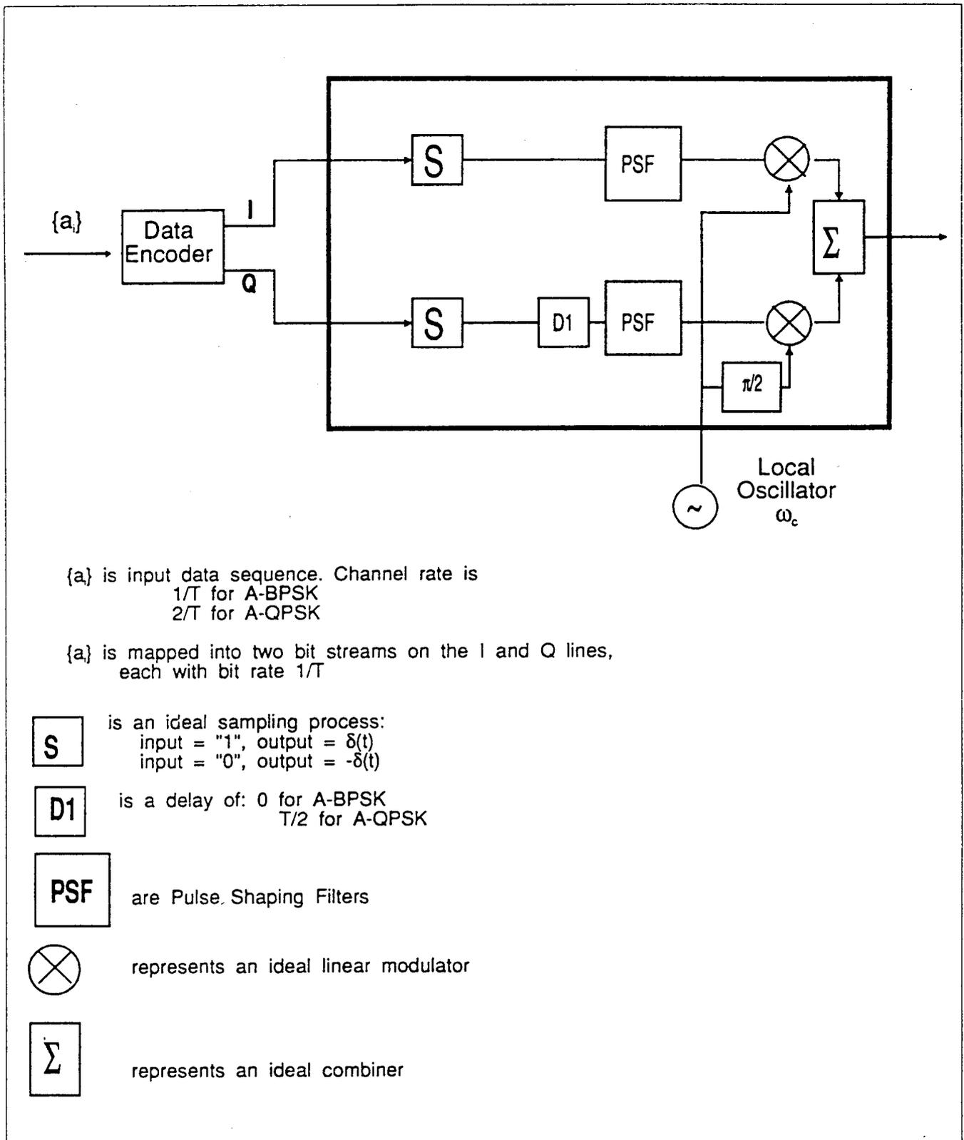
Figure A-4. Ideal modulator (A-BPSK and A-QPSK)
