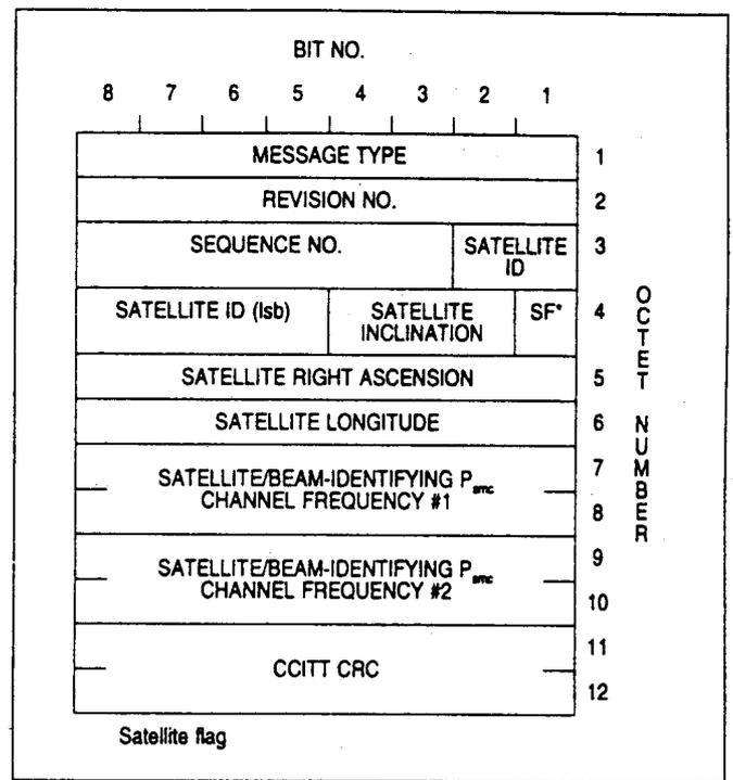
Figure A2-32. AES system table broadcast — P channel
