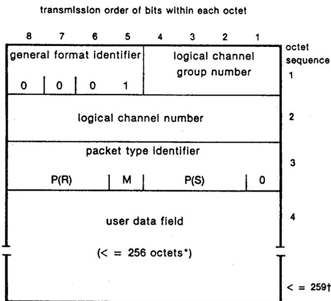
\* Data networks operating in the packet mode and connected with CIDIN using procedures described in ITU CCITT Recommendation X.25-1981 may limit the user data field to not more than 128 octets. Later versions of Recommendation X.25 will be reviewed as they are released to ascertain whether or not they should be adopted.
