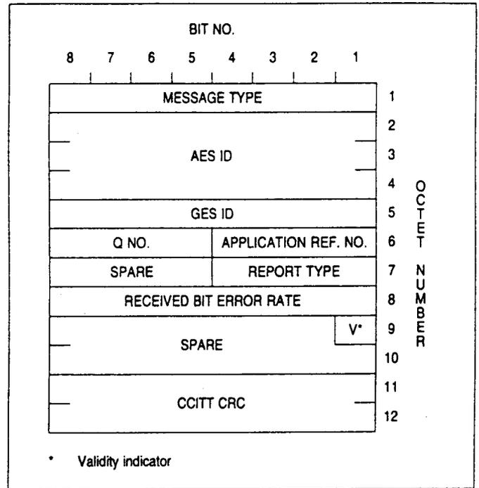
Figure A2-12. Call progress — from-aircraft sub-band C channel Channel status report
