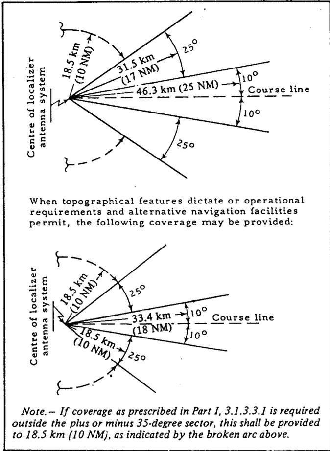
Figure C-7. Localizer coverage in respect to azimuth
