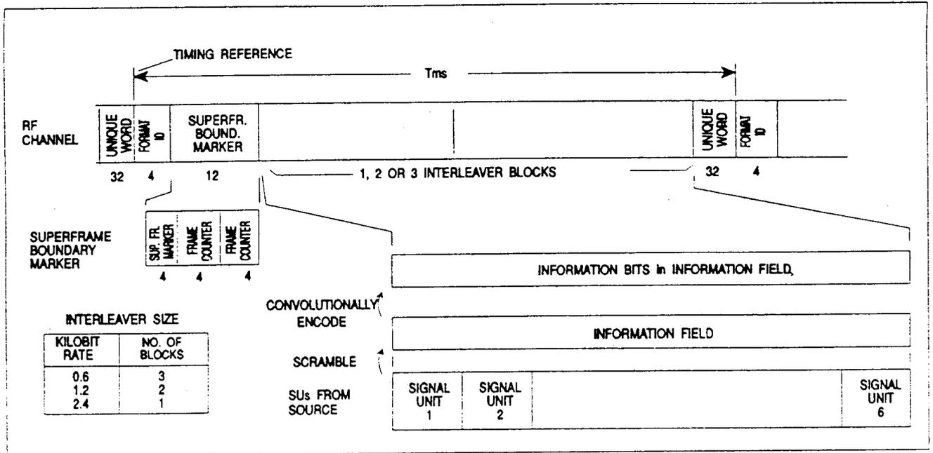
Figure 4-1. P channel format (0.6, 1.2 and 2.4 kbits/s)
