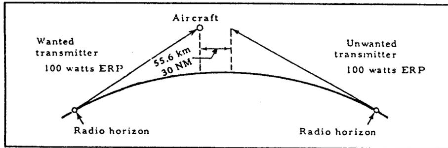
Figure A-5. VOLMET planning (illustrating co-channel protection)
