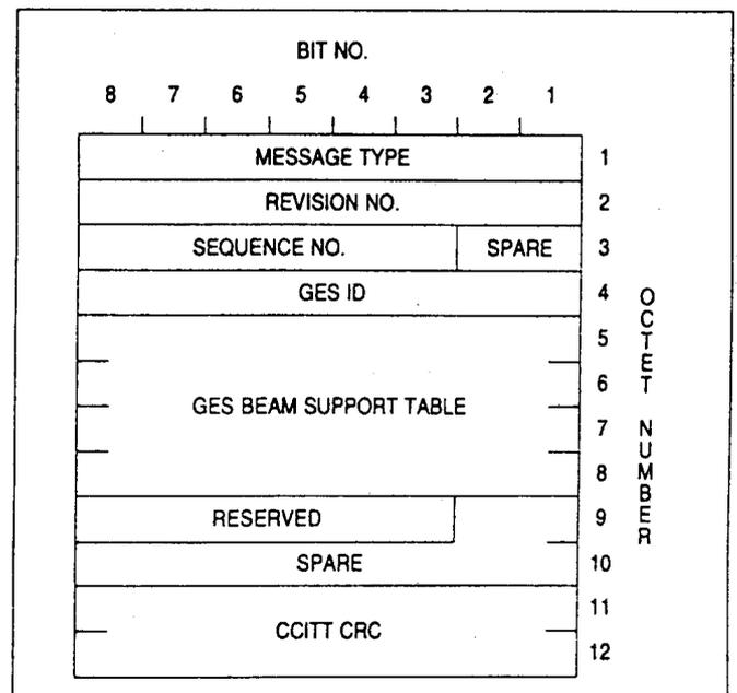
Figure A2-34. AES system table broadcast — P channel
