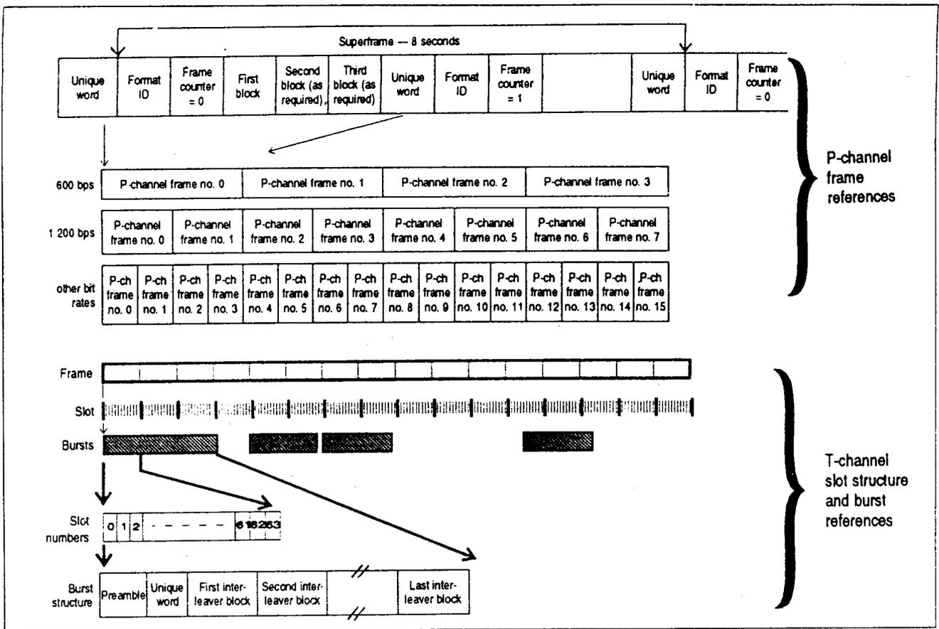
Figure 4-7. Timing references between P and T channels
