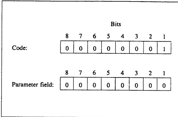
Figure 4-27. Fast select (use not permitted) facility format
