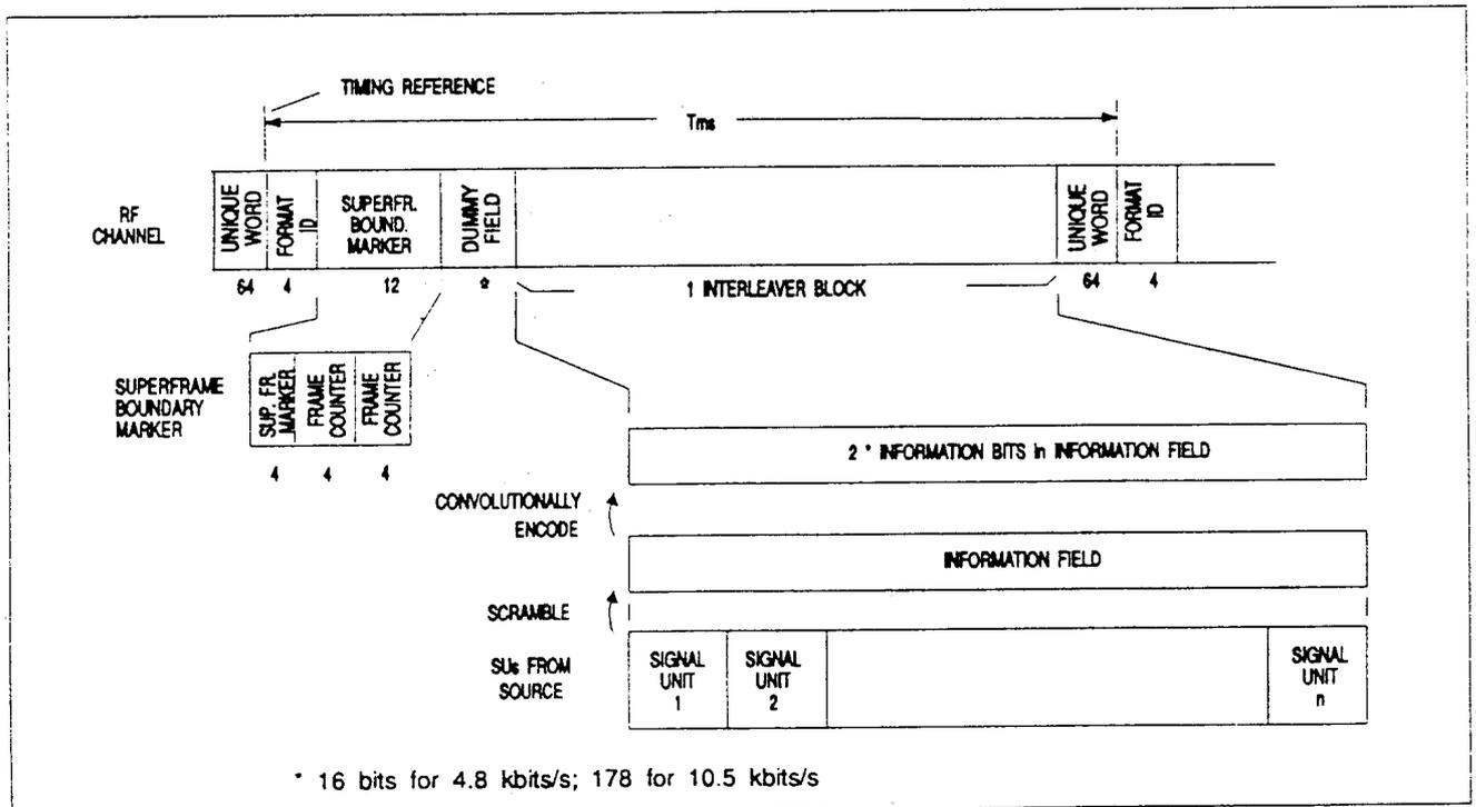
Figure 4-2. P channel format (4.8 and 10.5 kbits/s)
