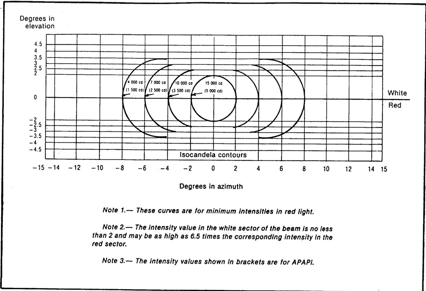
Figure 2.20 Light intensity distribution of PAPI and APAPI
